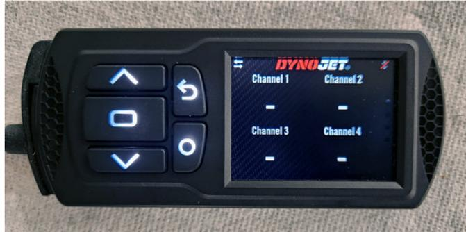
Your PV3 will probably power up at the gauges screen as shown above. Press the ENTER key to get to the main menu.
