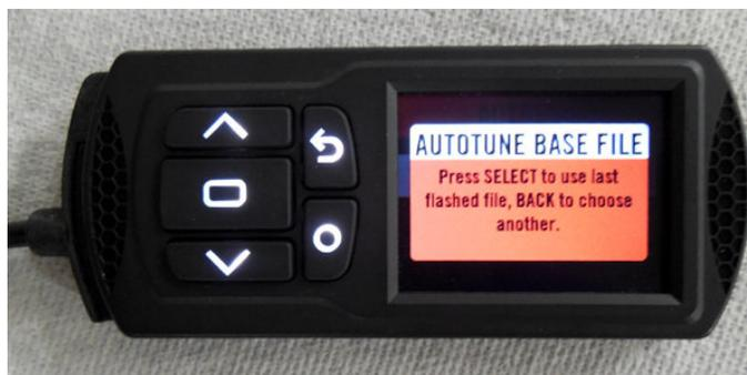
If you just want to build on the previously flashed tune, just press ENTER at this prompt. That will be the normal case. However, you do have the option of selecting a different tune as the basis for the auto tune section.
