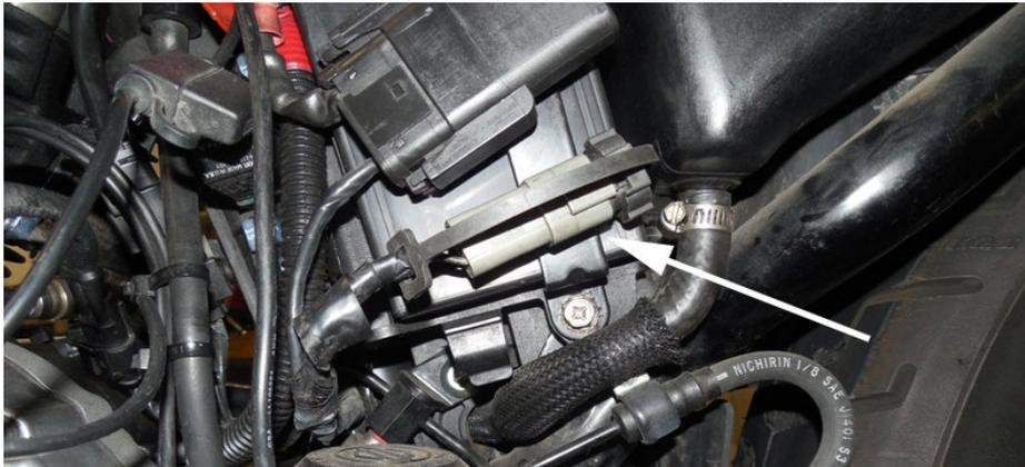
The diagnostic connector on a Sportster is found under the left side cover. Slide it up and to the right to free it, and remove the dust cap.
