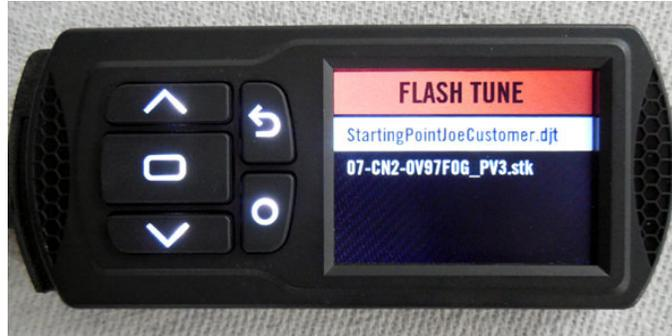
The above menu selections should be available. The .stk file is your bike's original tune, we don't want to flash that one. Instead, make sure the starting point tune we provided is selected as shown above and press the ENTER key.
