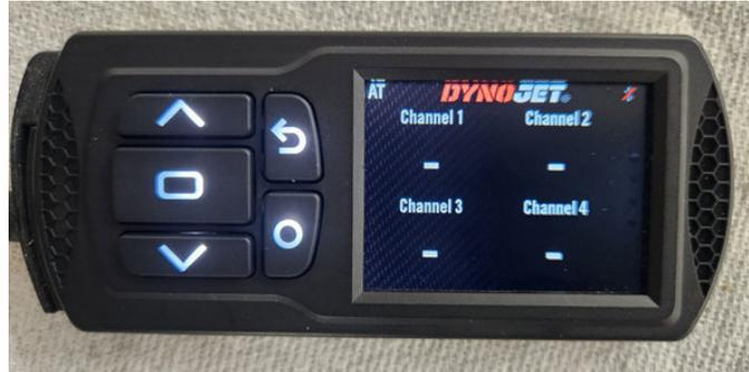
Notice the AT in the upper left corner, this is your indicator that you're in auto tune logging mode. When a smile face is next to it, it means logging is taking place. Logging won't take place unless the engine is up to temperature.
