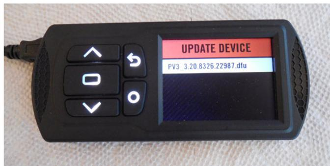
The new firmware file will appear as shown. If the PV3 firmware has been previously updated, other files may be shown. In that case, use the SCROLL buttons to highlight the new file. Now press ENTER.
