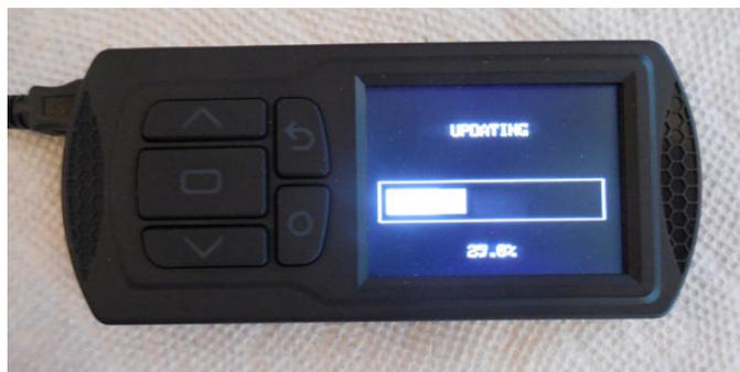
Various messages and progress bars will appear as the device updates its firmware. Do not unplug the USB cord or do anything else to remove power from the PV3 while this process is taking place.
