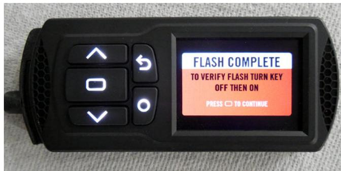
The PV3 will build a new tune, incorporating the learned values from your logging selection, and flash that tune to the bike as previously described. The above screen will be shown when the flash operation is complete.
