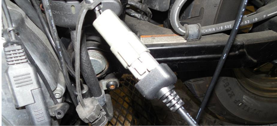
Plug the PV3's diagnostic cable into the bike's diagnostic connector as shown. The other end of this cable needs to be plugged into the PV3. Leave the PV3's USB cable disconnected.
