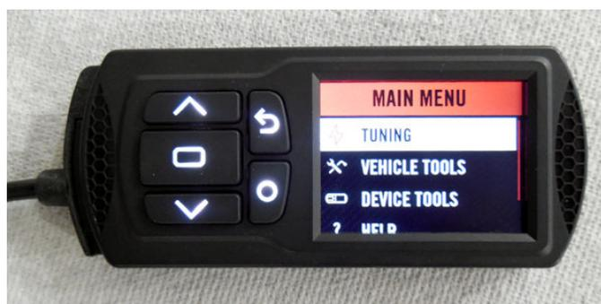
From the main menu, make sure TUNING is selected as shown above. Press the ENTER key to access the Tuning submenu.
